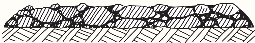
Single Otta Seal (0-16 mm). Thickness: minimum 16 mm
